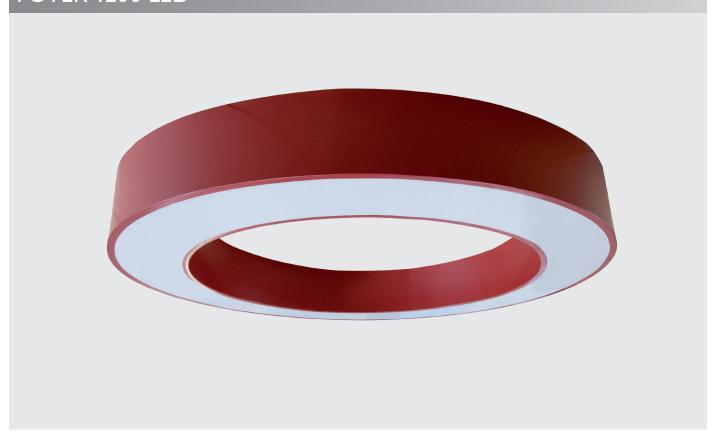
Suspended direct/indirect LED luminaires. Body is made of steel and aluminum and is available in all RAL colours. Light source - Philips, Osram or Tridonic LED module. Standard EVG ballast, DALI or Touch Dali version on request.
