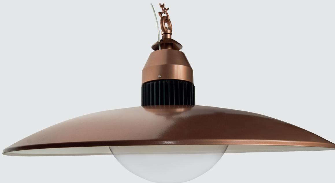
Pendent LED luminaire. Body is made of steel and aluminium and it is available in all RAL colours. Light source - Philips, Osram or Tridonic LED module. Standard EVG ballast, DALI or Touch Dali version on request. Standard length of suspension set - 1,5 meter:
