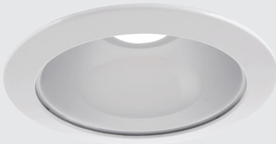
Recessed LED luminaire. Body is made of steel and aluminium and it is available in all RAL colours. Light source - Philips, Osram or Tridonic LED module. Standard EVG ballast, DALI or Touch Dali version on request. Passive cooling, optional IP44 diffuser.
