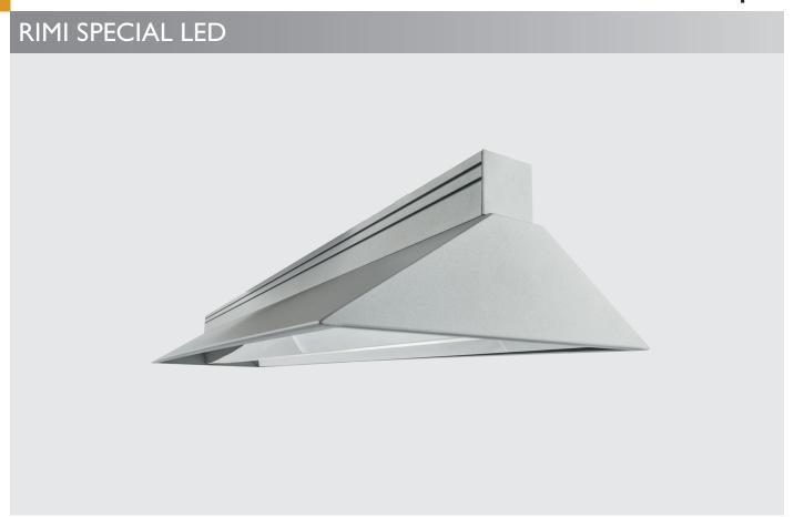
Pendent LED luminaire. Light source - Philips, Osram or Tridonic LED module. Standard EVG ballast, DALI or Touch Dali version on request. Body is made of steel and aluminium. Opal, acrylic or microprismatic diffuser. All RAL colours available. Different sizes on request.
